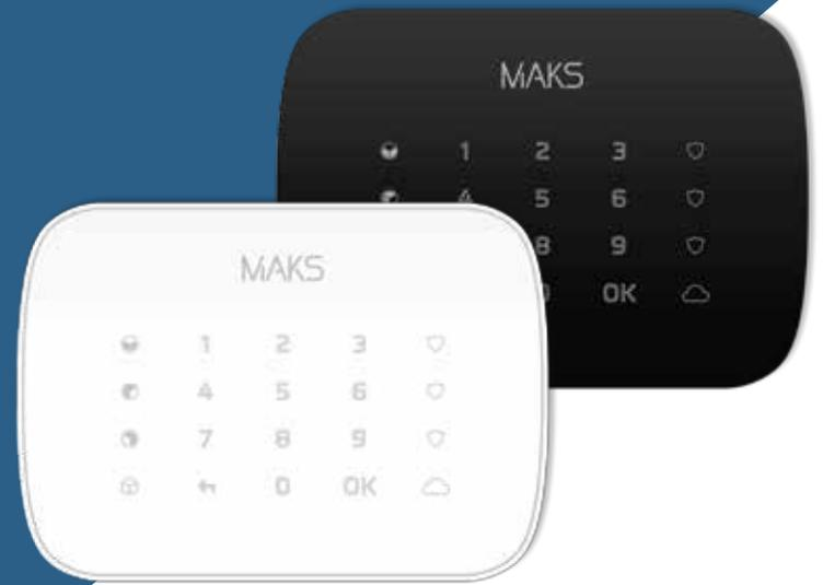
The wireless keypad is designed for arming and disarming, displaying alarms and device status, as well as interaction with the user of the alarm system.
